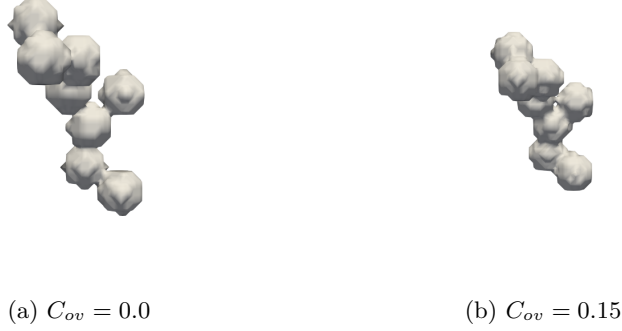
Figure 4: Example of two bare aggregates with N = 8 and D_f = 2.0 . a) aggregate with point-contacting monomers ( C_{ov} = 0.0 ) b) aggregate with overlapping monomers ( C_{ov} = 0.15 )
