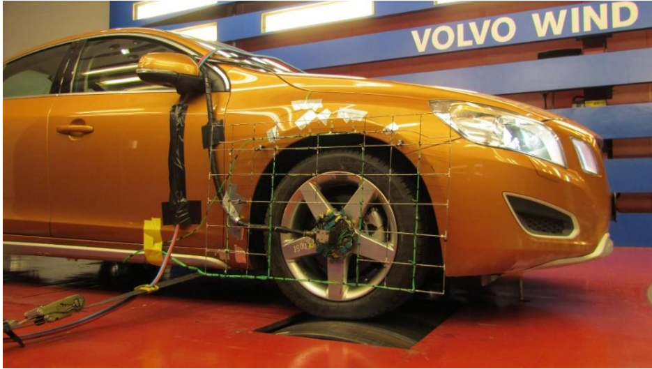
Figure 8. Vehicle positioned in the wind tunnel for the simulated Alpine Descent test
