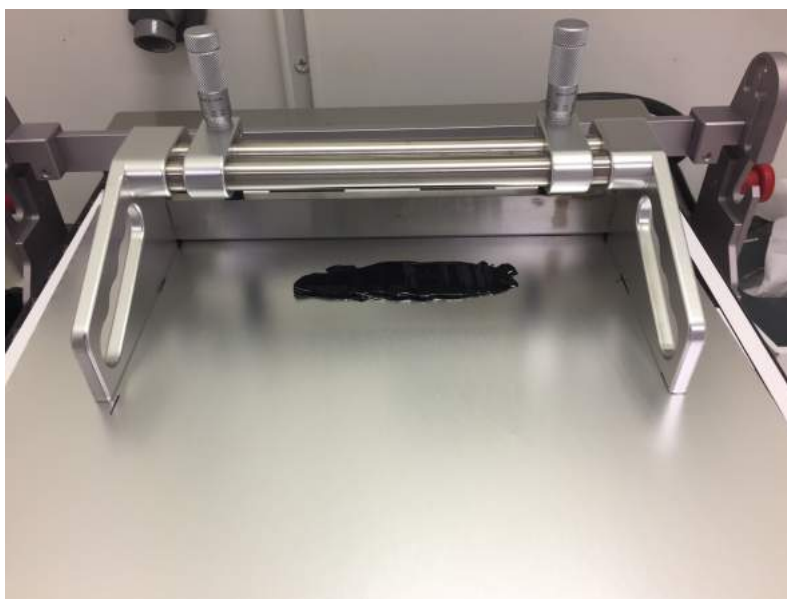
Figure 23. Picture of the doctor blade placed behind the carbon slurry just before coating.
