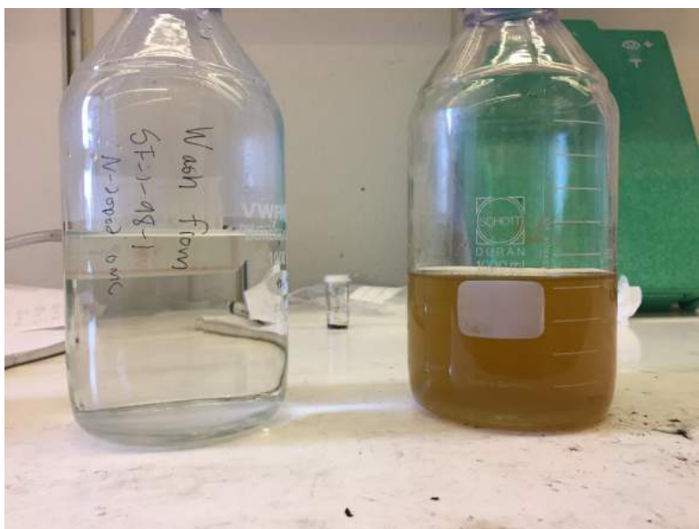
Figure 51. Picture of the filtrate after carbamate and DMF washes of the N-doped OMC (left) and the 75% \text{Cu}(\text{BF}_4)_2 doped OMC (right). The brown substance was believed to have been the non-porous surface layer.
