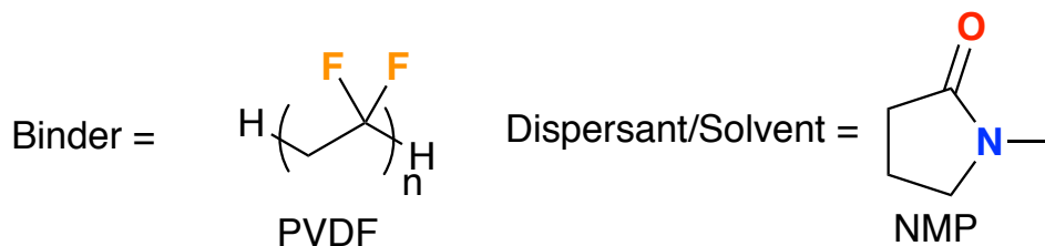
Figure 19. Chemical structures of the PVDF binder and NMP solvent/dispersant.
