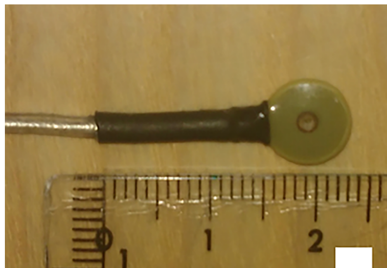
Fig 3. A localization coil used in the Elekta Neuromag TRIUX system (ruler scale is in cm).
