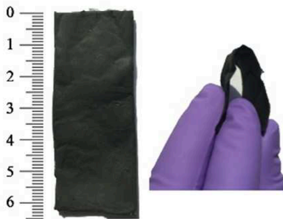
Figure 17. Self-standing carbon nano-fibre membrane prepared by electrospinning a PAN membrane followed by carbonization.
