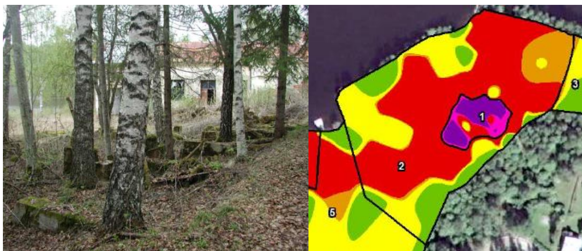
Figure 2-1. Left: Example of contaminated site. Remnants of the Kōja sawmill and the wood impregnation area. Right: Map of the interpolated dioxin levels within the former sawmill area, where the purple area shows the highest concentrations (>1500ng/kg TS) (Golder Associates, 2013).
