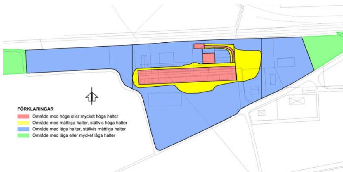
Figure 5-5. Assessed contamination levels at the BT Kemi southern site (from Sweco, 2011c). Green = low to very low levels; Blue=low to moderate levels; Yellow=moderate to high levels; Red=high to very high levels.
