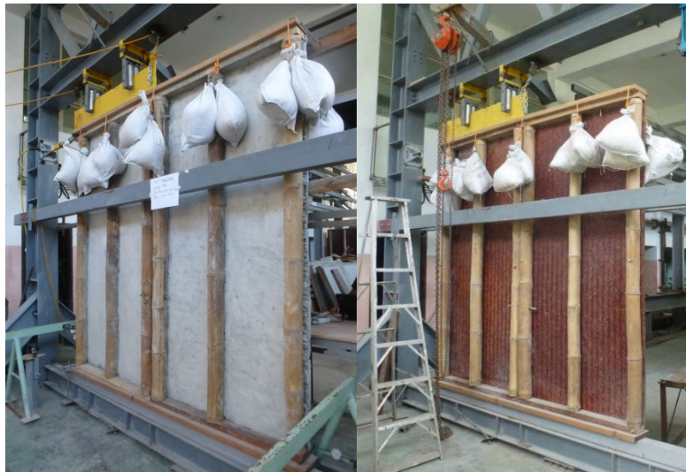
Figure 31 Racking strength tests of two kinds of bamboo frames
