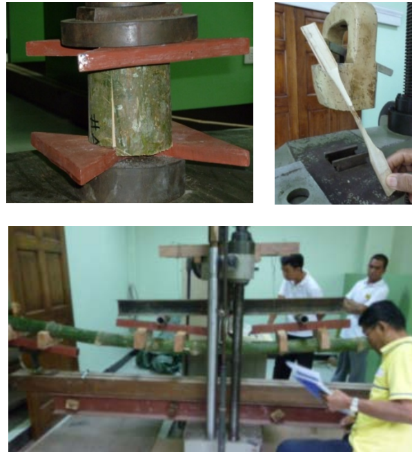
Figure 27 Shear, tension parallel and bending testing of B. blumeana
