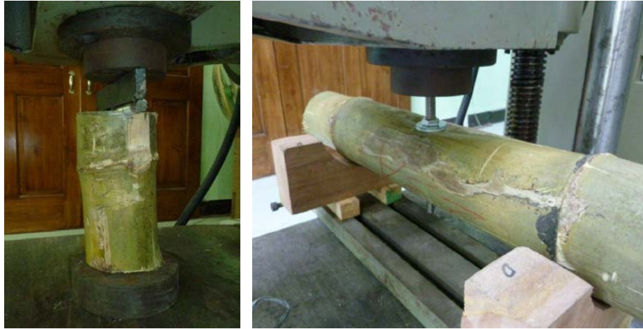
Figure 29 Embedment test (top left), and testing of connection types (right)
