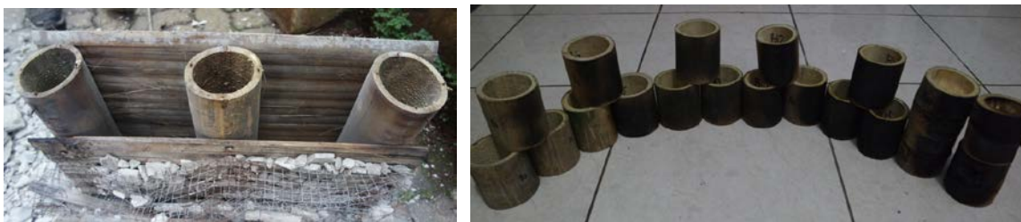
Figure 37 Bamboo cross-sections after test and classified according to charring rate
