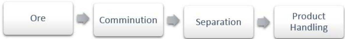
Figure 1. Principle flowsheet of the mineral processing stages.
