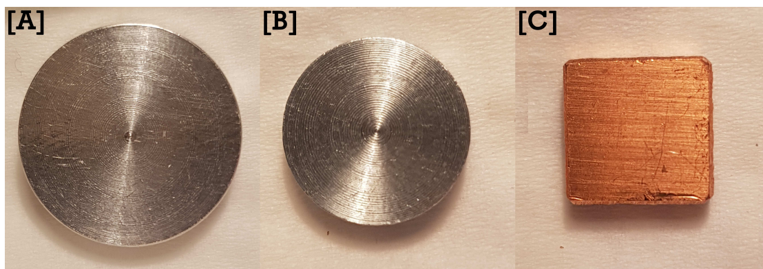
Figure 4. The general appearance of the coupon surface made from (A) aluminum, (B) zinc and (C) copper before being used in an experiment.
