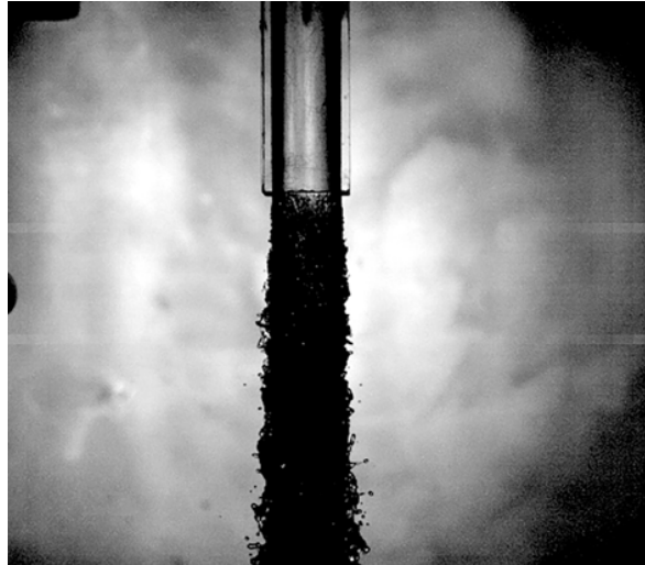
FIGURE 1. Image of near-field breakup in a 95% ethanol jet issuing from a 1 cm diameter nozzle at a bulk velocity of 15 \text{ m s}^{-1} , corresponding to Re = 72\,000 and We = 78\,000 .
