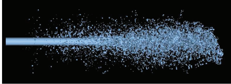
(a) The complete jet at t = 42.6 . The blue surface describes the isosurface of \alpha = 0.5 .
