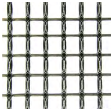
Figure 3.1: Carbon fiber mesh (SIGRATEX Grid 300) as anode material
