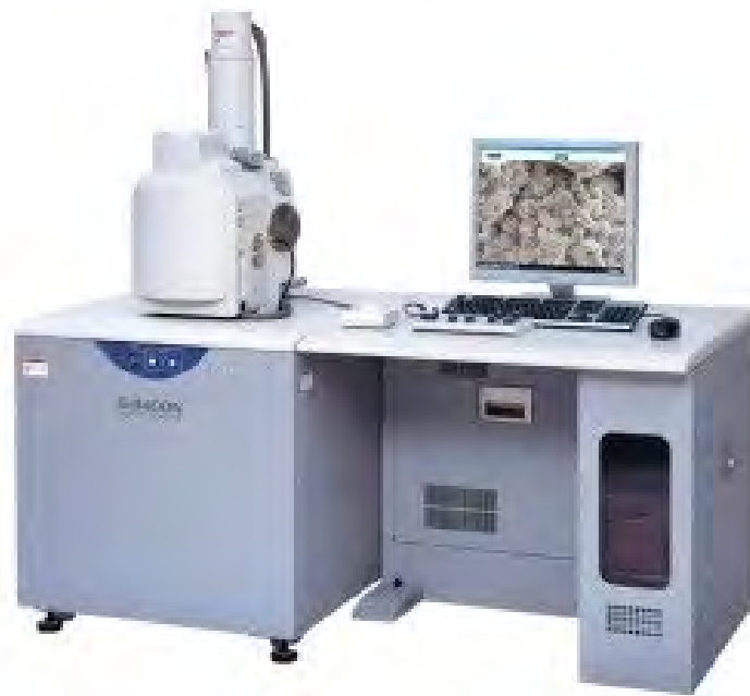
Figure 5.2: Hitachi S-3400N Variable Pressure SEM with EDS spectrometer
