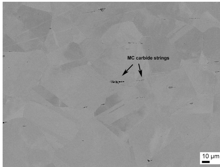
Figure 5: Microstructure of Haynes ® 282 ® in mill-annealed condition, with primary MC carbides visible as strings due to the manufacturing history [10] (Paper III).
