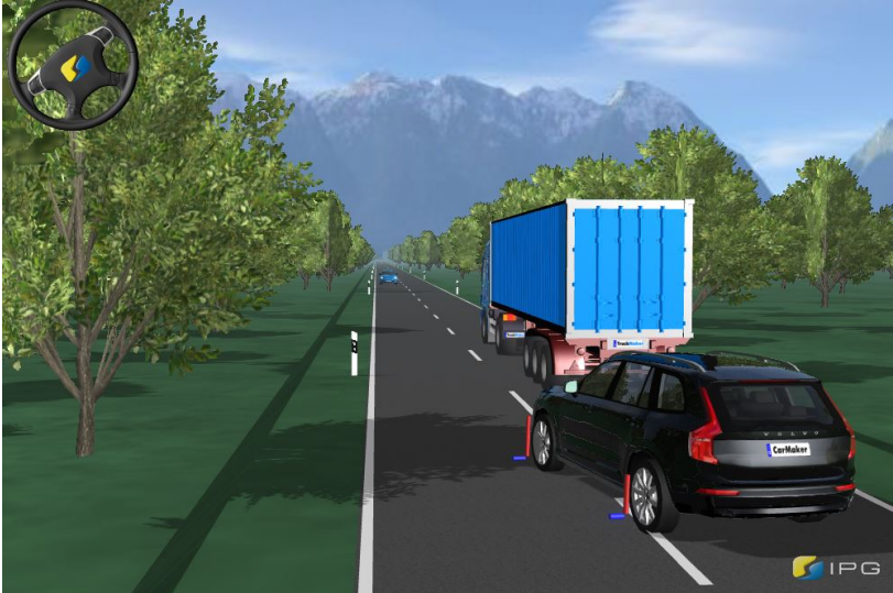
Figure 4.4: Screenshot of CarMaker simulation showing a scenario setup for the obstacle avoidance with oncoming traffic scenario. (figure reproduced from Paper E)
