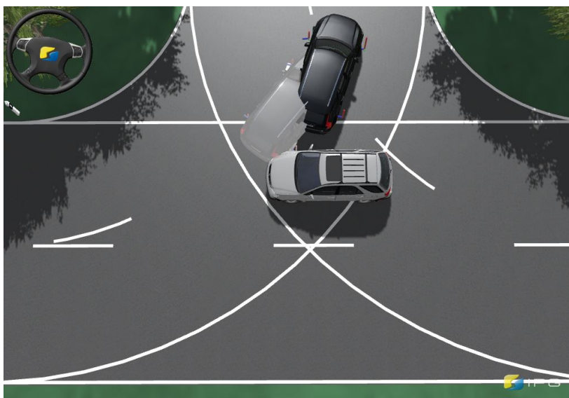
Figure 7.2: Screenshot of the host vehicle avoiding the bullet vehicle. The shaded host vehicle is the passive vehicle without an intervention. (image reproduced from Paper C)
