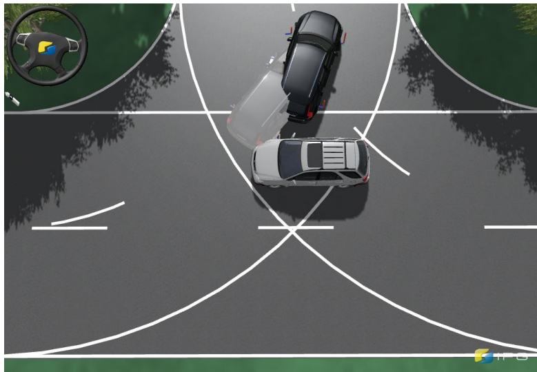
Figure 12 Screenshot of the host vehicle avoiding the bullet vehicle. The shaded host vehicle is the passive vehicle without an intervention.
