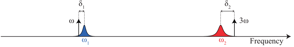
Figure 2.19: Frequency diagram indicating the first two modes of a \lambda/4 -resonator with positive anharmonicity, 3\omega_1 - \omega_2 > 0 . The arrows indicate a measurement signal, \omega and the drive signal at 3\omega . The measurement signal is placed at negative detuning \delta_1 , which results in a positive detuning \delta_2 .
