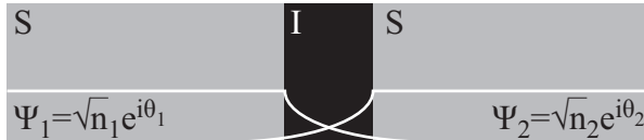
Figure 2.2: A superconductor-insulator-superconductor (SIS) junction. The white line indicates the BCS wavefunction, and the fact that the wavefunctions \Psi_1 and \Psi_2 overlap indicate that Cooper pairs can tunnel.
