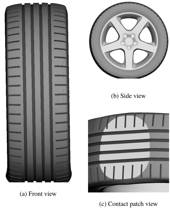
Figure 1: Tyre deformation under load on a passenger car.
