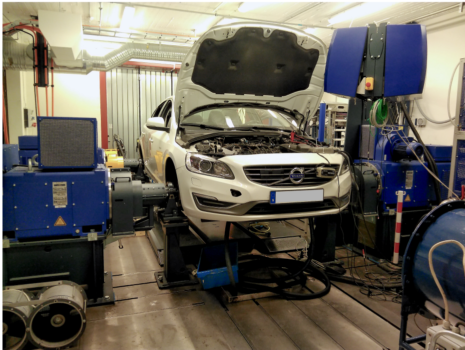
Figure 3.1: Test object installed in the test rig. Dynamometers attached to the wheels front and rear
