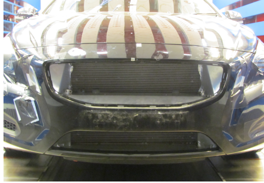
Figure 3.6: Reference configuration showing the aluminium ducts
