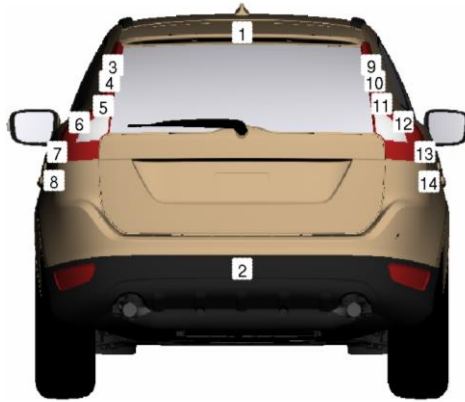
Figure 4. Locations of the unsteady pressure sensors mounted on the base perimeter.
