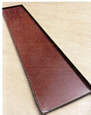
Fig. 6 Photo of collection trays that were placed in the driving gap under the window frame
