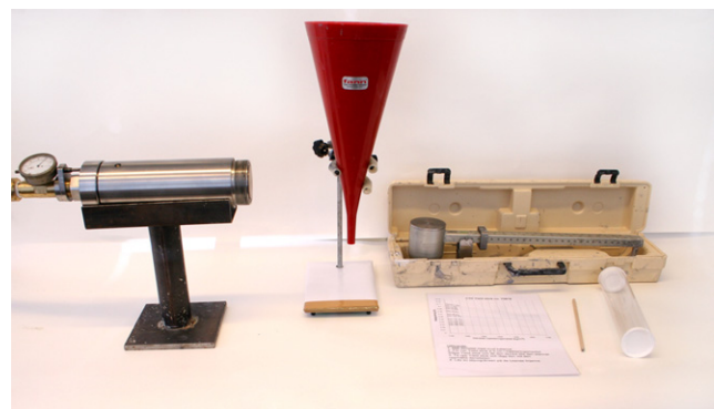
Figure 4. The four measurement devices. From the left, the PenetraCone, the Marsh funnel, the mud balance (at the back) and the yield stick, including the measurement graph (see also Figure 6) (picture by Nina Zanders)
