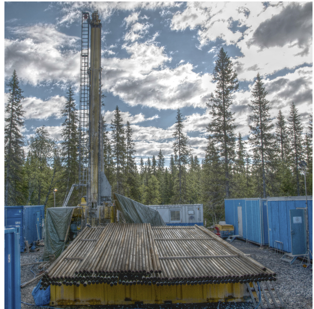
Figure 7. The Swedish national research infrastructure for scientific drilling, "Riksriggen". An Atlas Copco CT20C crawler mounted drill rig with a manual pipe handling system mounted on top of the mud tanks, with ca. 1400 m of HRQ drill pipe in this photograph.
