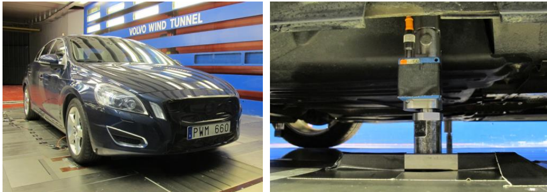
Figure 1. Overview of the wind tunnel model and displacement transducer attachment to the moving part of the floating strut.
