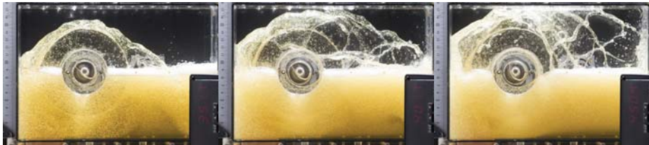
(d) Cylinder gear @ 350 RPM (e) Cylinder gear @ 400 RPM (f) Cylinder gear @ 450 RPM
