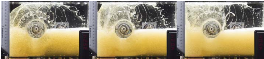
(a) FZG gear @ 350 RPM (b) FZG gear @ 400 RPM (c) FZG gear @ 450 RPM
