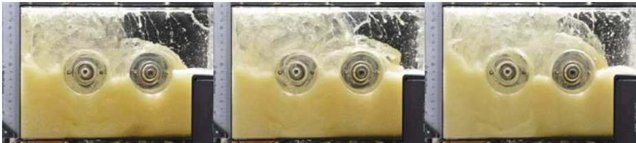
(g) FZG gear - Cylinder pinion @ 500 RPM (h) FZG gear - Cylinder pinion @ 550 RPM (i) FZG gear - Cylinder pinion @ 600 RPM
