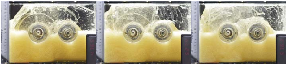
(j) Cylinder pair @ 500 RPM (k) Cylinder pair @ 550 RPM (l) Cylinder pair @ 600 RPM
