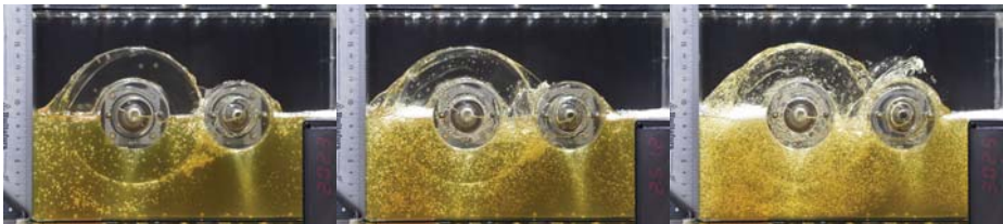
(j) Cylinder pair @ 200 RPM (k) Cylinder pair @ 250 RPM (l) Cylinder pair @ 300 RPM
