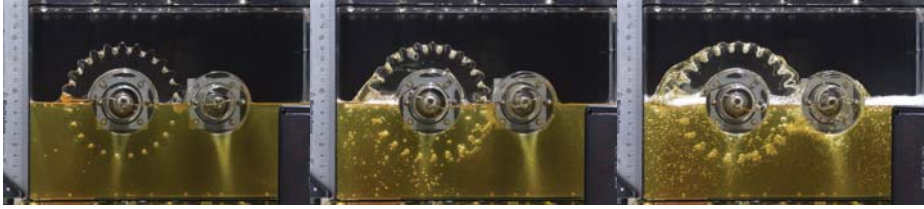
(a) FZG gear - Cylinder pinion @ 50 RPM (b) FZG gear - Cylinder pinion @ 100 RPM (c) FZG gear - Cylinder pinion @ 150 RPM
