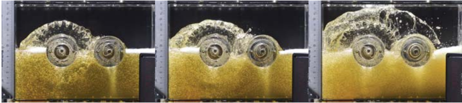
(g) FZG gear - Cylinder pinion @ 200 RPM (h) FZG gear - Cylinder pinion @ 250 RPM (i) FZG gear - Cylinder pinion @ 300 RPM
