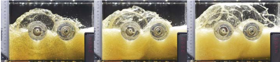
(d) Cylinder pair @ 350 RPM (e) Cylinder pair @ 400 RPM (f) Cylinder pair @ 450 RPM
