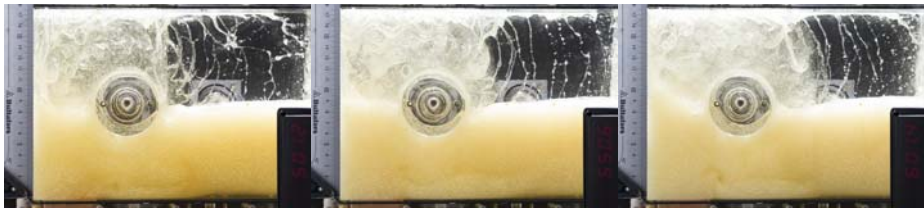
(g) FZG gear @ 500 RPM (h) FZG gear @ 550 RPM (i) FZG gear @ 600 RPM
