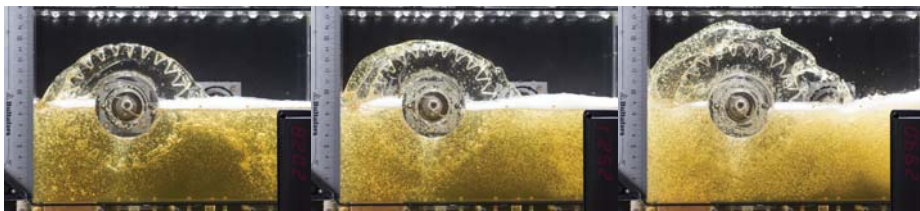
(g) FZG gear @ 200 RPM (h) FZG gear @ 250 RPM (i) FZG gear @ 300 RPM
