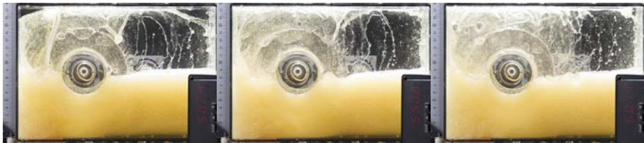
(j) Cylinder gear @ 500 RPM (k) Cylinder gear @ 550 RPM (l) Cylinder gear @ 600 RPM
