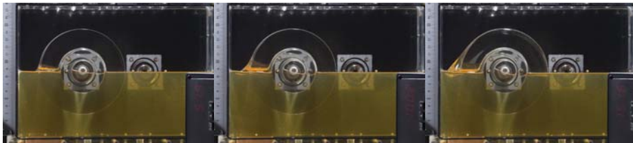
(d) Cylinder gear @ 50 RPM (e) Cylinder gear @ 100 RPM (f) Cylinder gear @ 150 RPM
