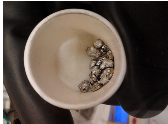
Figure 2. La-doped \text{Yb}_{14}\text{MnSb}_{11} crystals covered in a thin film of Sn. No crystals were big enough to enable measurement of Seebeck coefficient, electrical resistivity or thermal conductivity.
