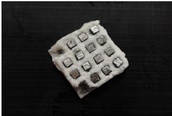
Figure 3. A grid is made out of an alumina paste and placed on the base plates. The thermoelectric materials is placed in a grid which keeps the legs in place and stabilizes the module when the top base plate has been placed.
