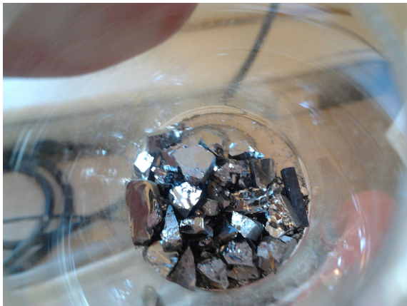
Figure 1. 20g of \text{Ba}_8\text{Ga}_{16}\text{Ge}_{30} single crystals. The size of the crystals was relatively consistent with some having a length of 1 cm making measurement of Seebeck coefficient and resistivity possible.
