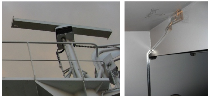
Fig. 4.3: Left: onboard wave radar (the navigation X-band radar) that measures the encountered waves. Right: deck longitudinal strain sensor at frame 179 on starboard side of the 2800TEU vessel. (Photos from Storhaug et al. (2007)).
